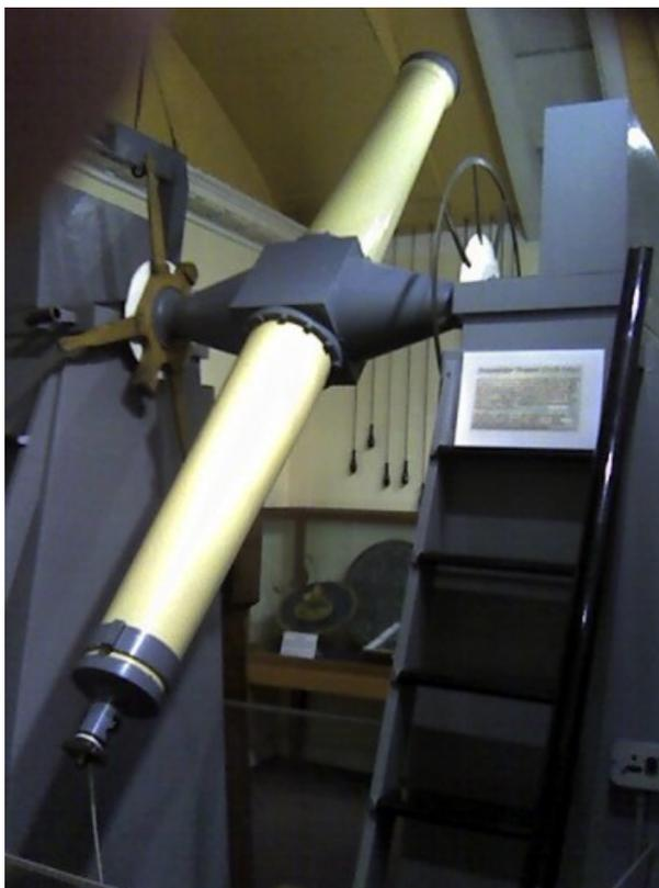
*The 160 mm Fraunhofer-Repsold Transit telescope
